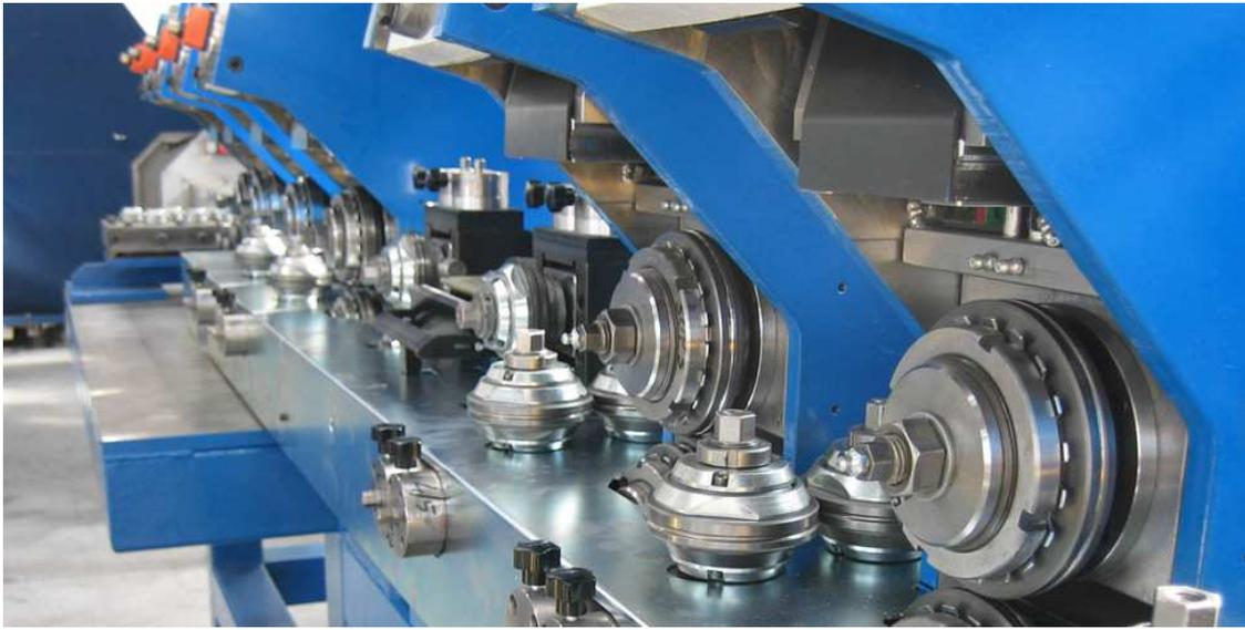
The fabrication of a Flux Cored Electrode begins by slitting steel coiled sheet into strips. The strips are passed through rollers that form it into a U-shaped cross-section. In the same operation, the formed strip is filled with a measured amount of core ingredients. The U-shaped strip is passed through closing rolls, forming it into a tube and tightly compressing the granular core material.
